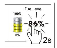
"Set fuel level at 100%" Once selected and confirmed *YES*, fuel level is set at 100%. Once selected and confirmed *YES*, fuel level is set to 100%.
