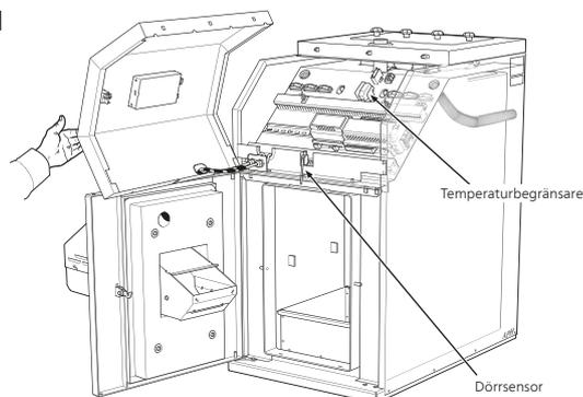
2. Disconnect the power supply to the boiler.
