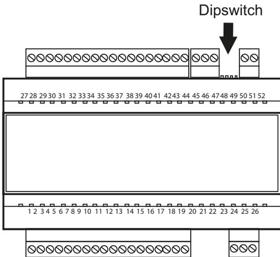
The switches are numbered 1 to 4. Switches 1, 2 and 3 are used to give the module a unique number. Switch 4 is for termination.
