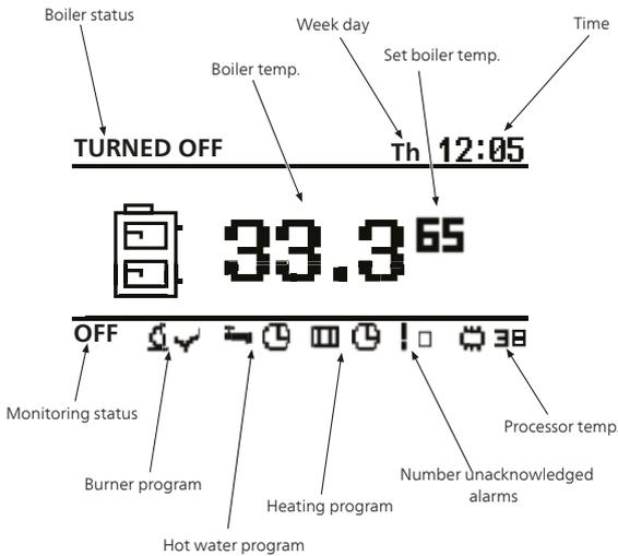
This is the menu that appears when PELLUX 100 is in its normal/start position. The menu displays boiler status, set temperature for the boiler and its current temperature. It is also possible to see the date, time, whether the control computer is being used or not, the running heating program, the number of alarms as well as the processor temperature.
