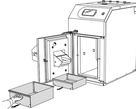
At the bottom of the hearth there is a removable ash box and a soot box. The ash box and soot box are generously sized and have room for ash and soot from two month's normal firing.
