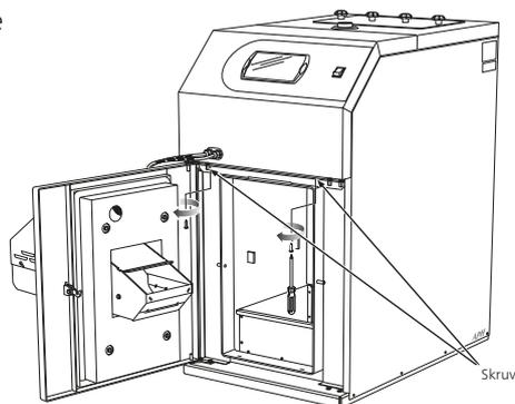
4. The front panel is held in place by catches. Pull the panel towards you and take care not to damage the cables connected to it.
