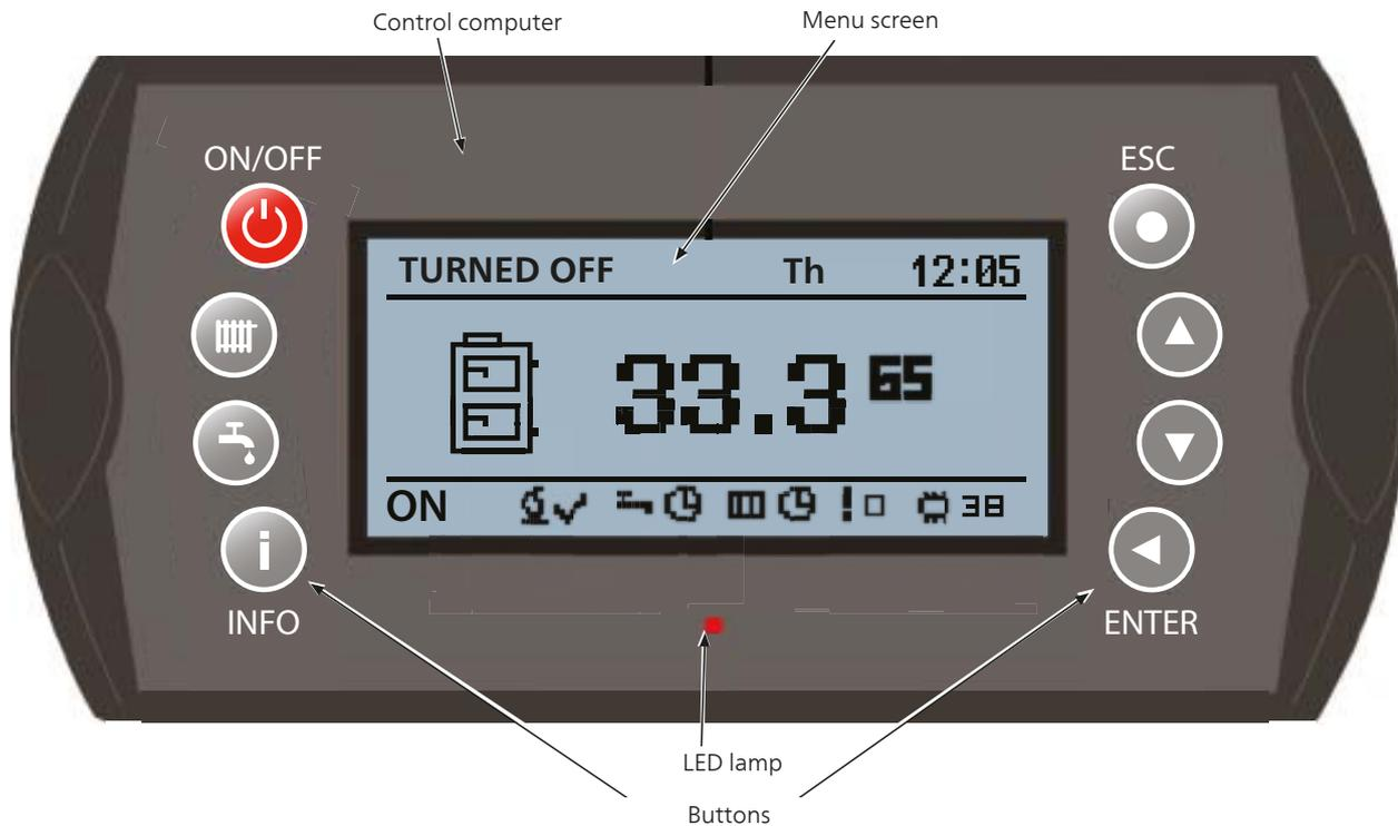
The control computer has two different menus that are displayed in the menu window:
