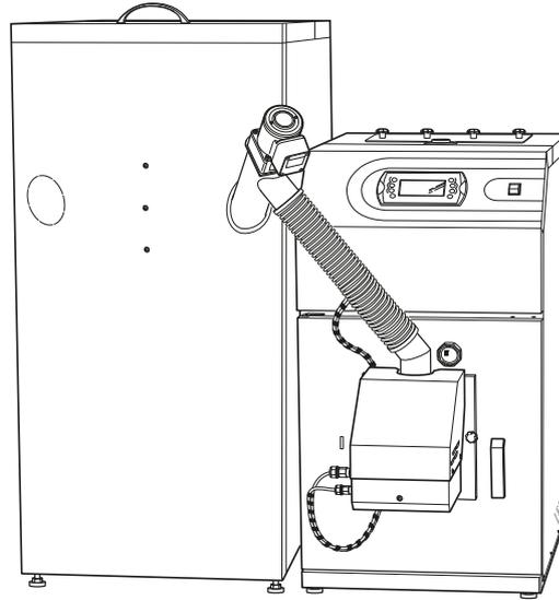
1. Position the pellet hopper in a suitable location and open the appropriate hole in the front.
