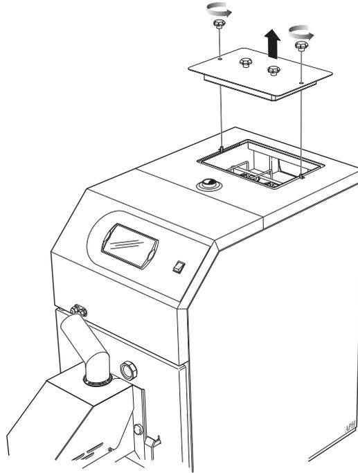
1. Open the soot hatches by slackening off the outer knobs.
