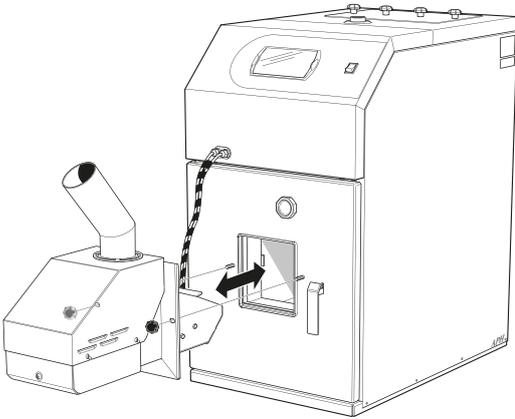
The burner is installed in the outlet for the burner on PELLUX 100s burner hatch. The burner is then secured into position using the knobs supplied for the burner.
