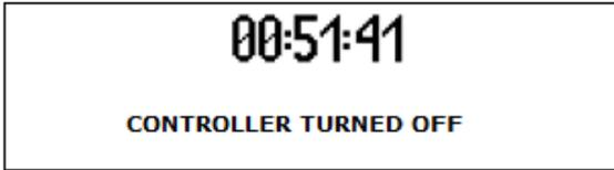
After pressing the ✓ button the controller menu will be displayed. To start the boiler, select "Turn on controller".
