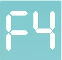
Open/Short circuit of outer tube temperature sensor: Dual-8 display shows **F4**
