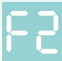
Open/Short circuit of inner tube temperature sensor: Dual-8 display shows **F2**
