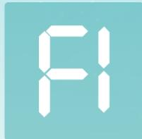
Open/Short circuit of ambient temperature sensor: Dual-8 display shows **F1**
