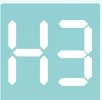
Overload protection:It will display **H3**(See overload protection function for more details)
