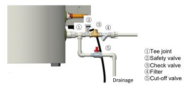
Installation Mode 2 of the Tap Water Valve (Inlet Water Pressure<0.1MPa)
