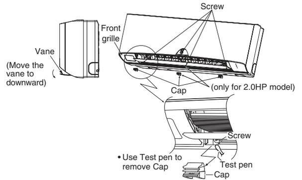
When reinstalling the front grille, carry out above step 2 - 3 in the reverse order.
