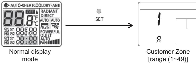
4 To enter Service zone: (Press SET continuously for T ≥ 5 secs)
